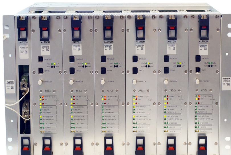
FIGURE II: Red Line & Orange Line Signals: Alstom’s AFTC-5 Digital Equipment to be Installed in Centralized Equipment Rooms
